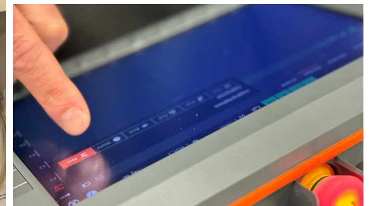
A symbiosis of robot and control unit: the KUKA smartPAD pro offers a wide range of features. The illuminated emergency stop is just one of them.
