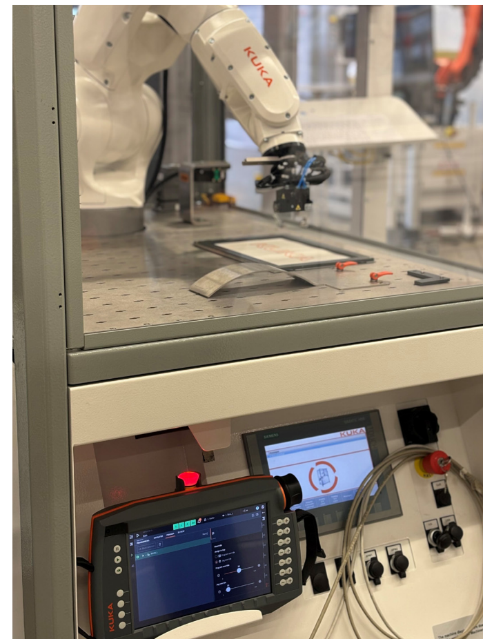
A symbiosis of robot and control unit: the KUKA smartPAD pro offers a wide range of features. The illuminated emergency stop is just one of them.
