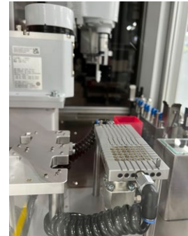
Figure 4: Automated application with vacuum pipette
