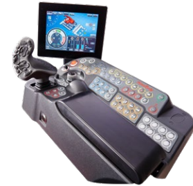
Figure 1: Example of armrest with complex RAFI joystick that measures a force when the joystick axis is rotated
