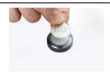
→ The RAFIX 22 FS+ FLEXLAB pushbutton allows individual control component labeling. A DIN A4 label sheet with pre-cut labels which fits in customary office laser printers is available for this option. After the legend inserts are printed, they be detached from the sheet and inserted into the colored lens using the fine stop tabs.
